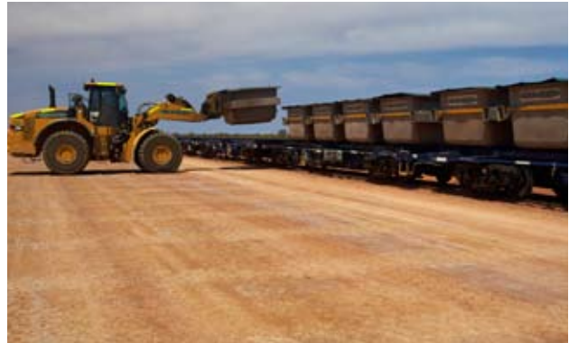
Loading kibbles onto a road train
